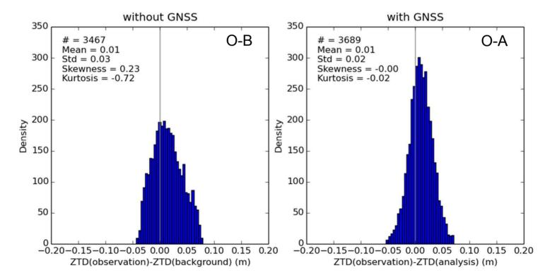
✓ The analyses of GNSS DA match the GNSS ZTD observations better than without GNSS cycle
