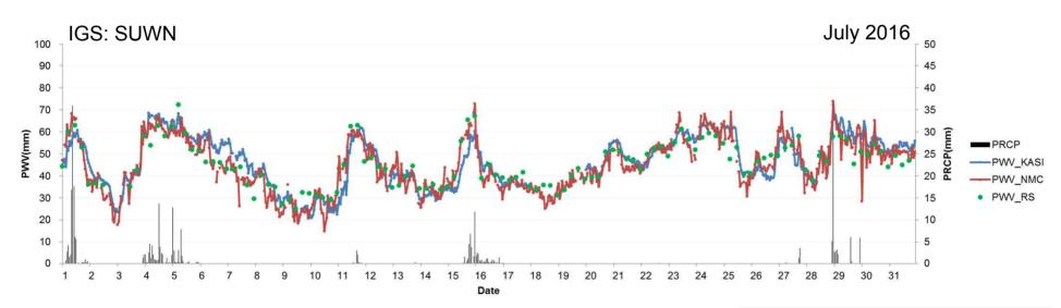
✓ Through comparison of the PWV with Sonde, the quality of GNSS data is reliable
